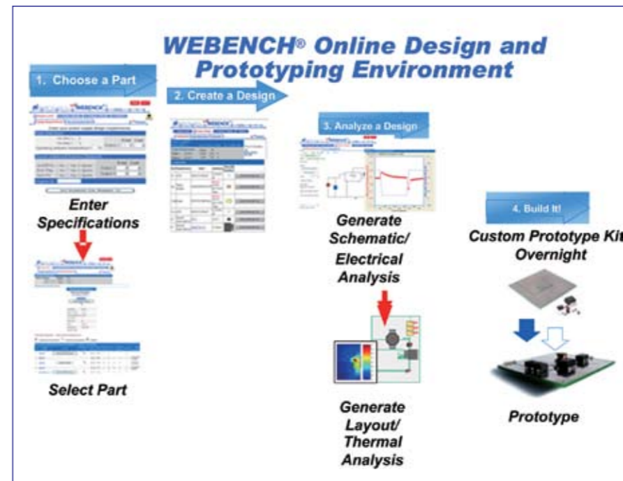
Figure 3: Webench on line tool: power supply design in four simple steps.
